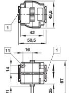
1 Main ports 1/4" or 3/8" ISO G/PTF Exhaust port M5 at 3/2 valve only
